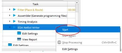
If the netlist creation was successful, run the gate-level simulation from the Tools menu
